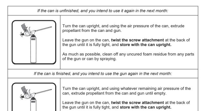
As much as possible, clean off any uncured foam residue from any parts of the gun or can by spraying.
